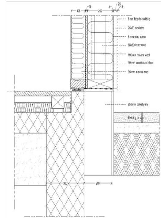
Cross section floor slab/wall. 200 mm x 400 mm insulation has been added to the base of the building to reduce thermal bridge effects. In addition to reducing the heat loss this has also raised the temperature of the floor and thereby improved the indoor climate. Now the entire floor area is useable for the occupants.
