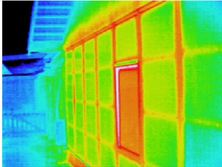
*Left: Thermography before renovation. Notice how the beams in the existing wall and the frame of the window create large thermal bridges. Also the window itself is showing a significant heat loss.*
