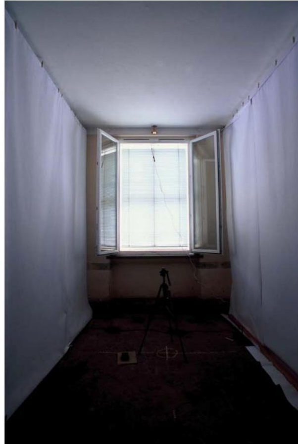
exterior and interior glazing: double low-E; shading system: Blinds: Warema Genius E 50 (white)
