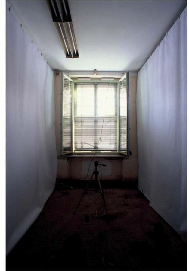
exterior and interior glazing: double low-E; shading system: Blinds: Warema Genius C/E 50 (mirrored aluminum)
