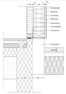
Cross section floor slab/wall. 200 mm x 400 mm insulation has been added to the base of the building to reduce thermal bridge effects. In addition to reducing the heat loss this has also raised the temperature of the floor and thereby improved the indoor climate. Now the entire floor area is useable for the occupants.
