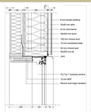
Cross section window/wall joint. The existing insulation of 95 mm have been replaced and a new layer of 195 mm insulation have been added to the exterior wall. The window has been moved out in the construction. The original thermal bridges in the wall and the thermal bridge at the joint are reduced significantly.
