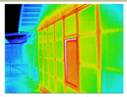
Left: Thermography before renovation. Notice how the beams in the existing wall and the frame of the window create large thermal bridges. Also the window itself is showing a significant heat loss.
